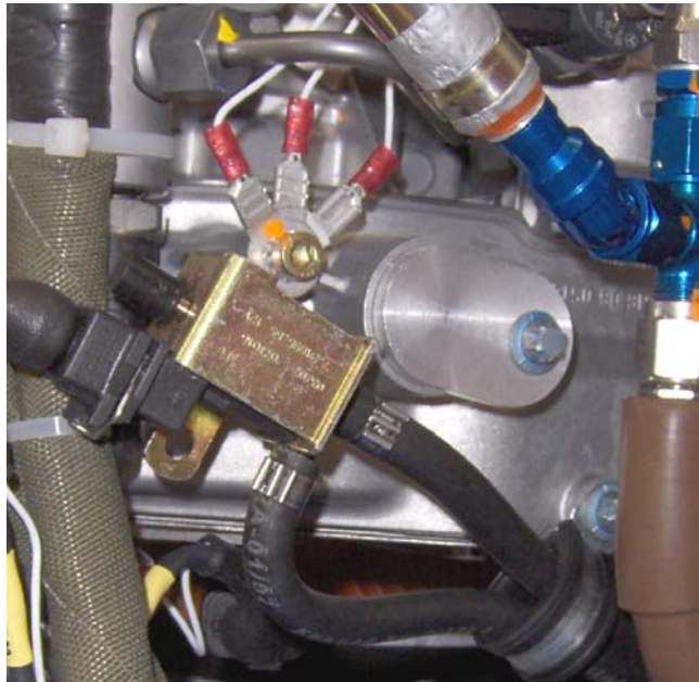
Bild 1/ Figure 1 Montage des Boost Regelventil ohne Befestigungslasche (P/N 57.81.07.010) Installation of boost control valve without the support lug (P/N 57.81.07.010)
